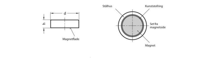
d =  $13 \pm 0,1$ h =  $4,5 \pm 0,2/-0,1$ Holding force N = 10Material = HF hard ferrite -  $200^{\circ}$  C
